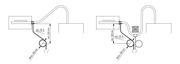
Lead the condensate hose down with a **minimum slope of 20** %, in the form of a **siphon (min. hose bend diameter Ø200 mm)**, directly into a discharge funnel.
