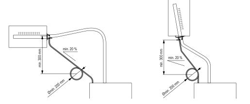
Lead the condensate hose down to the humidifier with a **minimum slope of 20** %, in the form of a **siphon (min. hose bend diameter Ø200 mm )**. Then, lead the hose into the unit through the break-through on the top side of the unit and insert it about 2 cm into the specified opening of the water cup.
