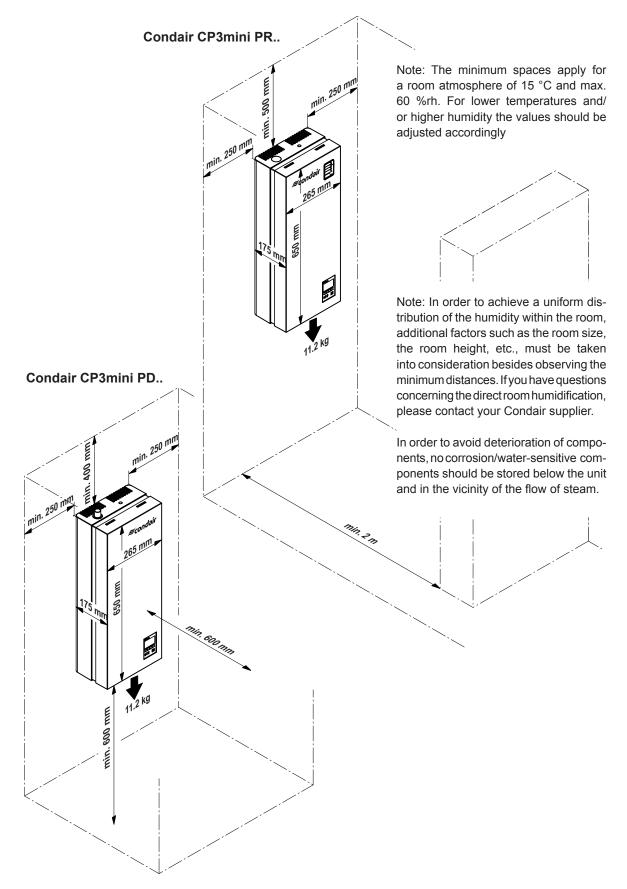
To **ensure proper functioning** of the steam humidifier and to **obtain an optimal efficiency**, the following points must be considered and observed when choosing the location for the steam humidifier:
