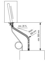
Initially, lead the steam hose with an **upslope of at least 20% over a minimum height of 300 mm** above the top edge of the unit, then lead the hose with a **minimum upslope of 20%** and/or a **minimum downslope of 5%** to the steam distribution pipe.
