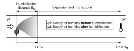
The calculation of the humidification distance " $B_N$ " is dependent on several factors. For a rough estimation of the humidification distance " $B_N$ ", the following table is useful. Recommended standard values listed in this table are based on a supply-air temperature range of 15 °C to 30 °C.
