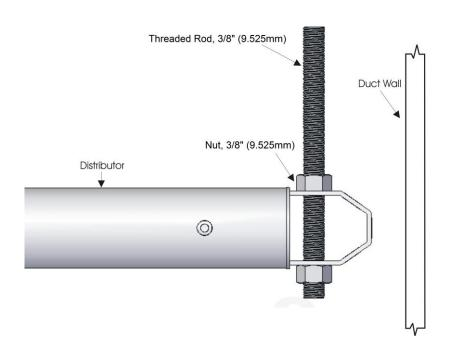
Figure 14: Duct Support Bracket with Horizontal Duct Wall
