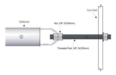
Figure 12: Duct Support Bracket Away from Duct Wall
