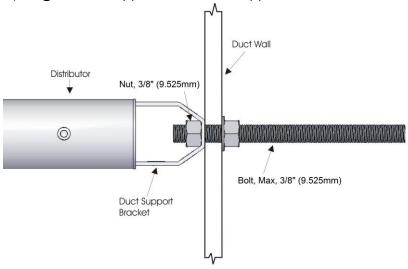
Figure 11: Duct Support Bracket Flush with Duct Wall
