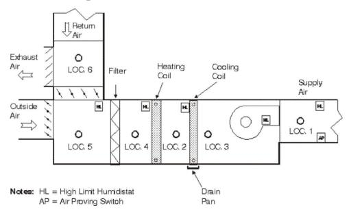
Figure 2: Air Handling Unit
