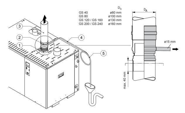
1 Flue gas connection on the unit
