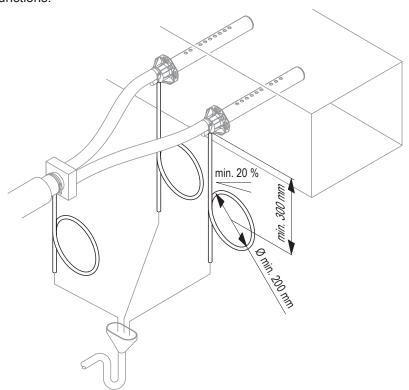
The individual condensate hoses of the main steam pipe (if present), the steam hose adapter (if present) and the steam distribution pipes must be led down with a **minimum downslope of 20** % via a siphon (min. hose bend ø200 mm) into a discharge funnel.
