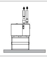
Note: Where local regulations permit, the RS units can be installed as C63x appliances. As a C63x appliance, the Condair GS can be connected to a separately approved and maketed system for the supply of combustion air and discharge of flue gases. For such applications, refer to the applicable local regulations and the separate Installation Instructions "Installation as a C6 appliance" available from your Condair dealer.
