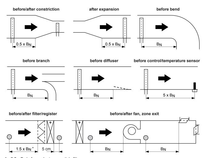
2,5 x B<sub>N</sub> before submicron particle filter
