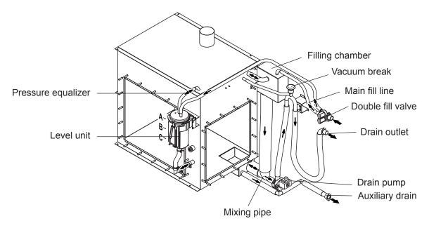
The level in the water tank is continuously monitored by the level unit. On initial start-up, the control unit checks the function of the level unit. During this test the tank is filled up first to level "A", then drained to level "C" and filled up again to level "A". As soon as level "B" is reached and the test of the level unit was successful the humidifier is ready for operation, if a humidification demand is present the combustion process starts.
