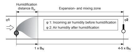
The calculation of the humidification distance " $B_N$ " is dependent on several factors. For a rough estimation of the humidification distance " $B_N$ ", the following table is useful. Recommended **standard values** listed in this table are based on a supply-air temperature range of 15°C to 30°C. The values given **in bold print only apply to steam distribution pipes 81-..**, the **values in brackets apply to the OptiSorp steam distribution system**.
