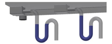
The air-lock need to have a height of minimum 30 mm in order to compensate for pressure difference and prevent air from being sucked in through the air lock.
