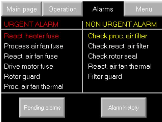
Fig. 6: Alarms submenu
